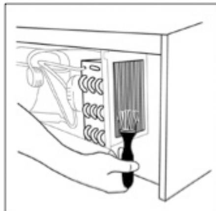
Fig. 2: Cleaning the condenser with a brush and vacuum cleaner in a refrigerated cabinet
