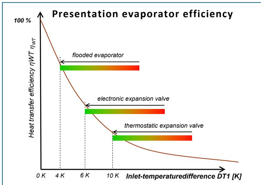
Fig. 4: Evaporator efficiency chart (source: VDMA 24247-8)
